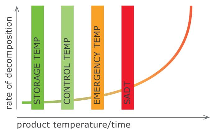
Controlling the temperature is the most important constant. If the temperature is maintained well below its self-accelerating decomposition temperature (SADT), most hazards are avoided when shipping, handling or storing. For storage over a longer period of time, follow the manufacturer's temperature recommendations.
